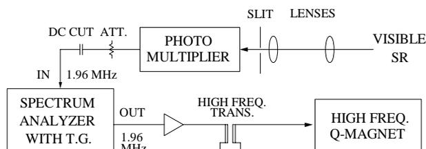
Figure 1: Setup for the horizontal quadrupolar tune measurement.
