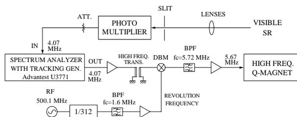
Figure 2: Setup for the vertical quadrupolar tune measurement.
