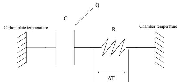
Figure 2: Equivalent circuit of the BIHM.
