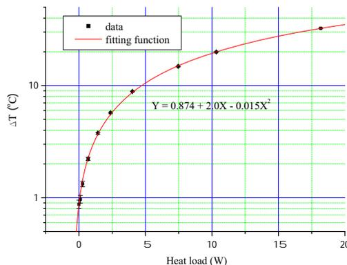
Figure 4: Sum of the equilibrium  $\Delta T$  signals as a function of the heat load of the heater. The error bars are the standard deviation obtained from the data
