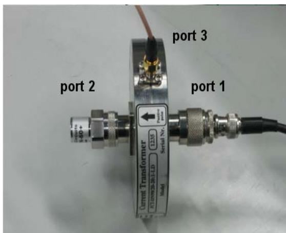
Figure 2: Tuned current transformer.
