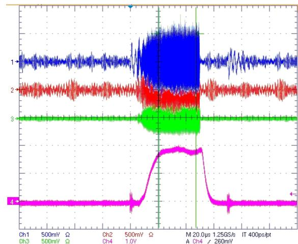
Figure 3: Measured beam current - 2mA peak (Ch 1 : RFQ output current, Ch2 : tank2 output current, Ch 3 : tank3 output current, Ch4 : 20 MeV DTL output current)
