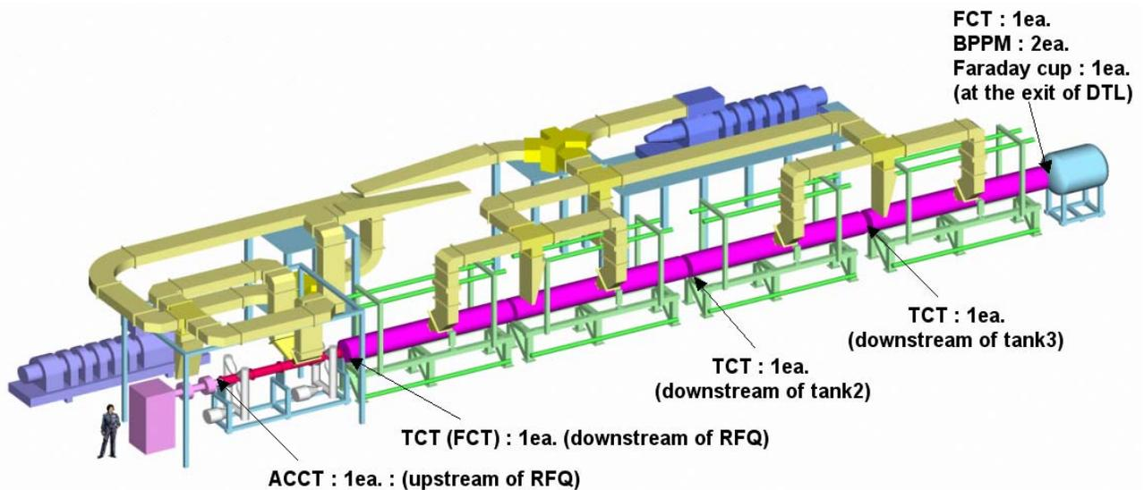
Figure 1: Beam diagnostics layout.
