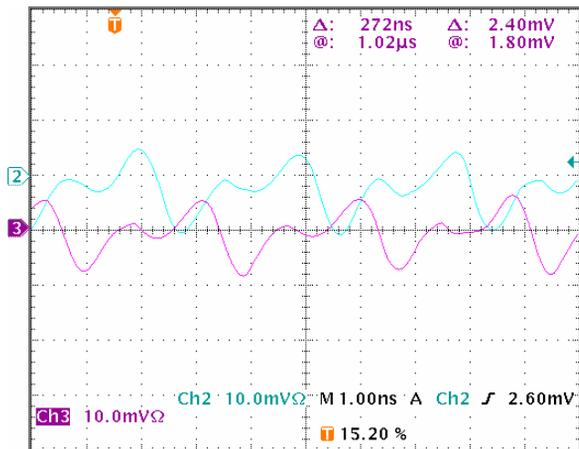
Figure 4: Measured BPPM signal (Ch 1 : upstream side - BPPM1, Ch 2 : downstream side – BPPM2)
