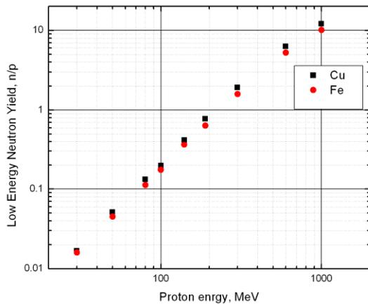
Figure 5. Calculated neutron yield from copper and iron targets.
