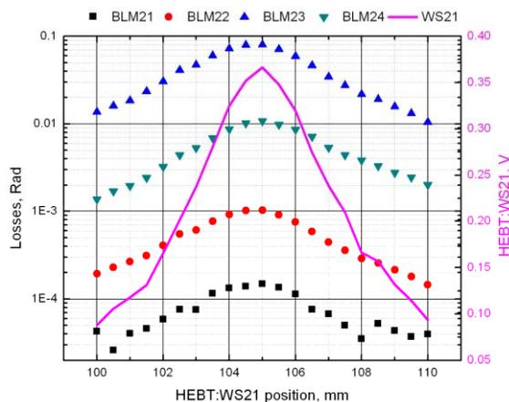
Figure 6. BLM signals correlate with WS position
