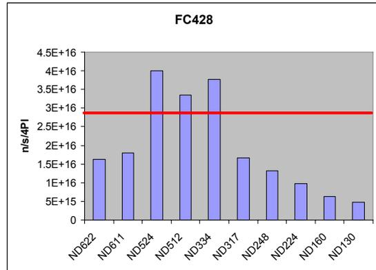
Figure 4. The calculated neutron intensity (red line) and measured results (blue bars)
