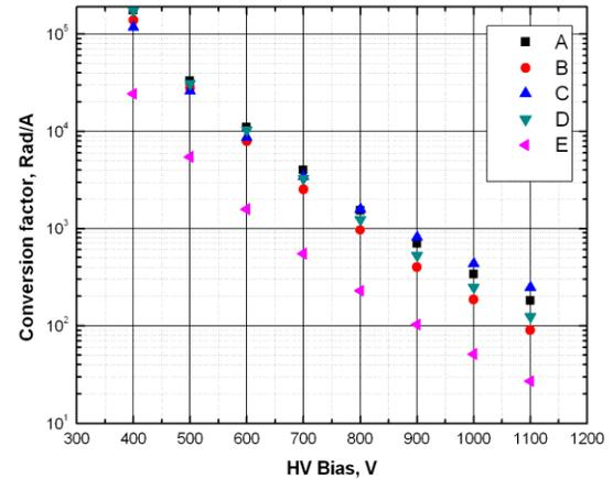
Figure 1: Typical HV dependence for NDs
