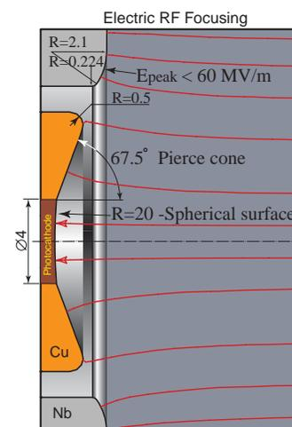
Figure 1: View of the photo cathode stem disposed into the hole of the back cavity wall of the RF gun. The electric field of the image charge in the entire wall was taken into account in the calculations. The optimized sizes are presented in the picture.
