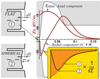
Figure 2: Cathode geometry and accelerating field distribution along the axis of a 1 cell RF gun cavity for  $r=1$  mm.
