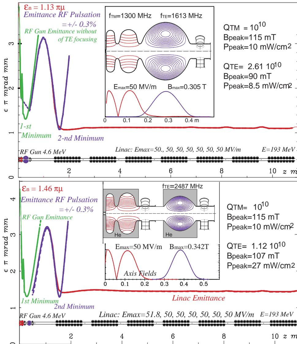
Figure 4: Transverse normalized emittance of bunches in a superconducting 1.5 cell photo cathode RF gun and in a linac with TESLA cavities. The electric RF focusing is shown in fig. 1. The RF power feed for the TM mode has to be made from the side of the cathode assembly. The RF peak power density at the surface for the TE mode ( $P_{peak}$ ) is close to the TM mode peak density.
