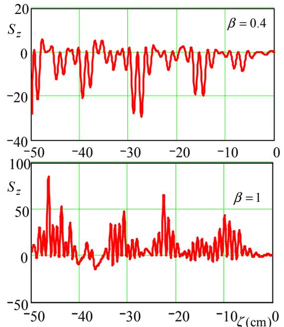
Figure 3: Amplitudes of magnetic components of harmonics and z-projection of energy flow density on the waveguide boundary for the same parameters as in Fig.2 and  $q = 10^{-12} C$  (SI-units).
