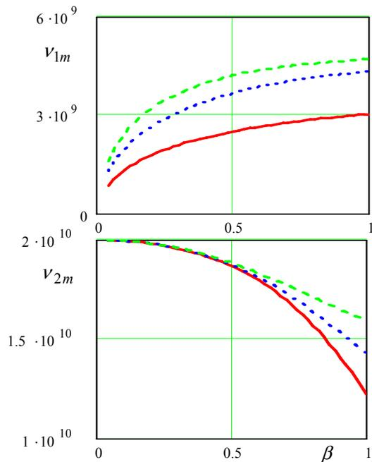
Figure 2: Frequencies of three modes ( $m=1,2,3$  correspond to the solid, dotted, and dashed curves accordingly) of the 1<sup>st</sup> and 2<sup>nd</sup> series for a waveguide with bi-anisotropic medium:  $v_{re} = 0$ ,  $v_{pe} = 5$  GHz,  $F = 0.5$ ,  $v_{rm} = 20$  GHz,  $v_{de} = v_{dm} = 0$ ,  $a = 3$  cm.
