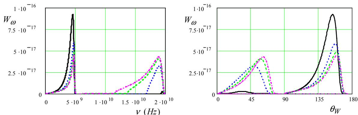
Figure 1: Spectral density of radiated energy per unit area (in SI-units) depending on frequency and angle. Magnitudes of parameters are the following:  $v_{re} = 0$ ,  $v_{pe} = 5 \text{ GHz}$ ,  $v_{rm} = 20 \text{ GHz}$ ,  $F = 0.5$ ,  $v_{de} = v_{dm} = 10^{-2} \text{ GHz}$ ;  $\rho = 10 \text{ cm}$ ;  $q = 10^{-12} \text{ pC}$ ;  $\beta = 0.4$  (solid),  $\beta = 0.7$  (dotted),  $\beta = 0.9$  (dashed),  $\beta = 1$  (dash-dotted).
