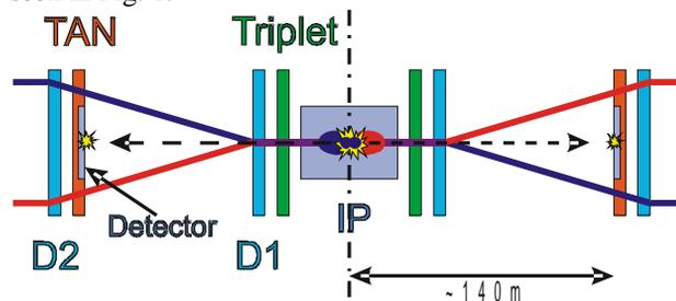
Figure 1: Typical layout of a luminous IR in LHC.
