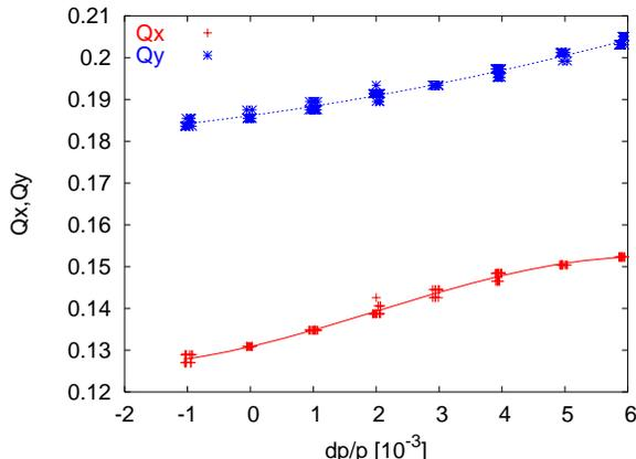
Figure 3: Tunes versus relative momentum deviation from the 2006 experiment at 26 GeV and  $1.1 \times 10^{10}$  ppb together with a fit.
