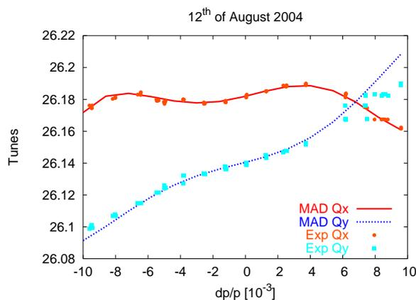
Figure 2: Tunes versus relative momentum deviation from the 2004 experiment at 26 GeV and  $4 \times 10^{10}$  ppb together with the matched model.
