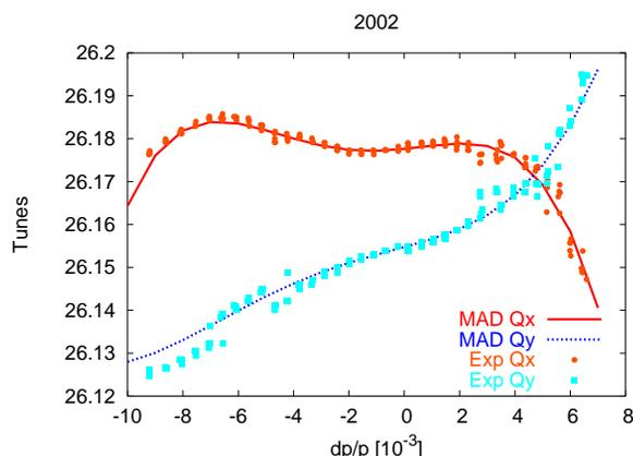
Figure 1: Tunes versus relative momentum deviation from the 2002 experiment at 26 GeV and  $4 \times 10^{10}$  ppb together with the matched model.
