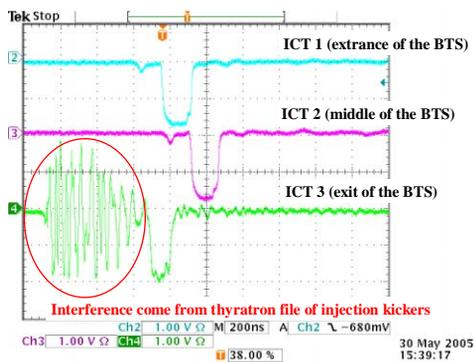
Figure 3: The ICT3 signal suffers the interference during injection kickers fired.
