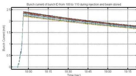
Figure 7: Ten consecutive bunch current of in decay mode operation.
