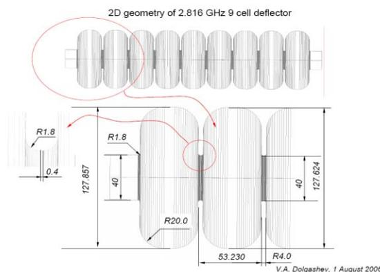
Figure 2: A 2.816-GHz 9-cell deflecting cavity.
