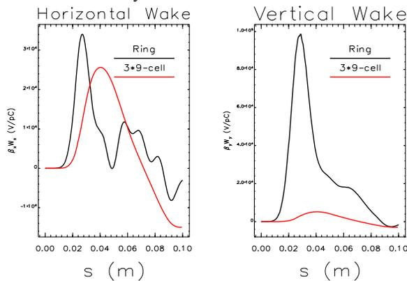
Figure 3: Comparison of a total wake potential of the ring and three 9-cell cavities: horizontal wake  $\beta_x W_x$  (left) and  $\beta_y W_y$  (right).
