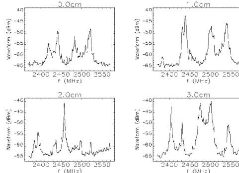
Figure 5: Horizontal scraper HOMs vs. inserted position.
