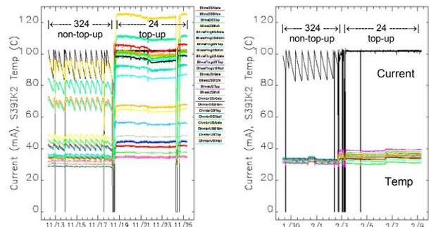
Figure 1: Kicker chamber temperatures before (left) and after (right) redesign (two-week period each, 100 mA).
