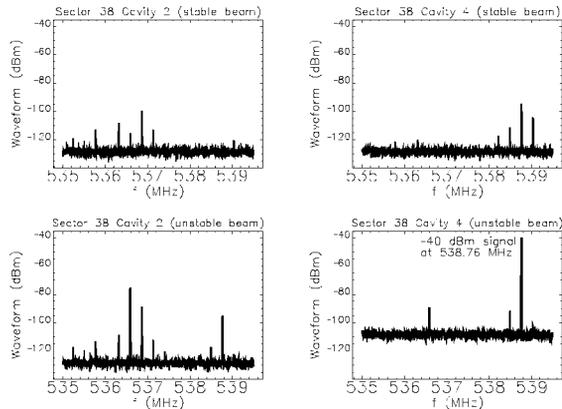
Figure 2: HOM spectra for cavities 2 and 4 in sector 38 for stable (top) and unstable (bottom) conditions (24 bunches, 100 mA) prior to installation of the dampers.
