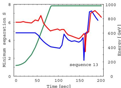
Figure 2: Beam separation during ramp and squeeze presently (red) and in the beginning of Run II (blue).
