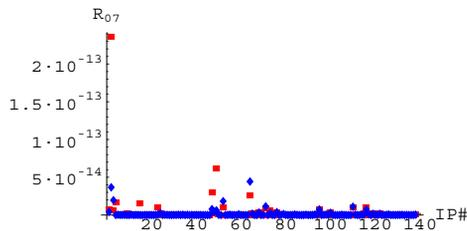
Figure 5: IPs contribution to the  $7Q_y$  RDT with beam separation shown in Fig. 4
