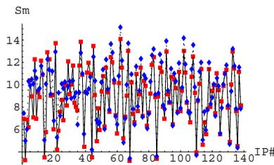
Figure 4: Beam separation at injection vs IP number with present (blue) and May 2002 (red) helices.
