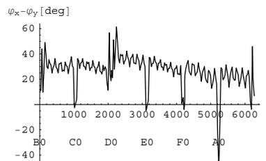
Figure 3: Phase advance difference around the ring starting from B0 with injection optics.
