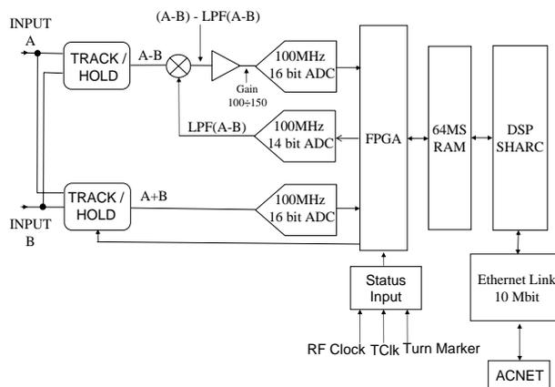
Figure 1: Schematic of the Digital Tune Monitor.
