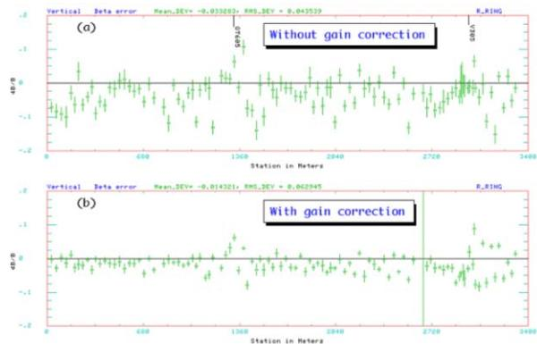
Figure 6: Results of vertical beta function measurement and plotted as  $\Delta\beta/\beta$ . In plot (a) is the case without applying gain calibration and plot (b) with gain calibration. The measurement is based on 1-bump closed orbit with multiple corrector dipoles, not the TBT analysis as mentioned.
