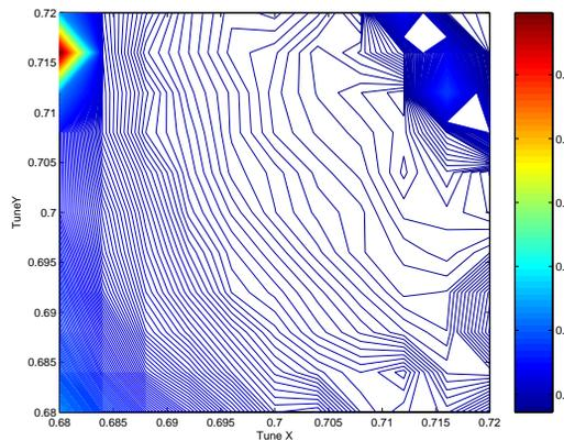
Figure 5: Averaged emittance growth as a function of betatron tunes for 4 sigma and 6 sigma separation including tune modulation.
