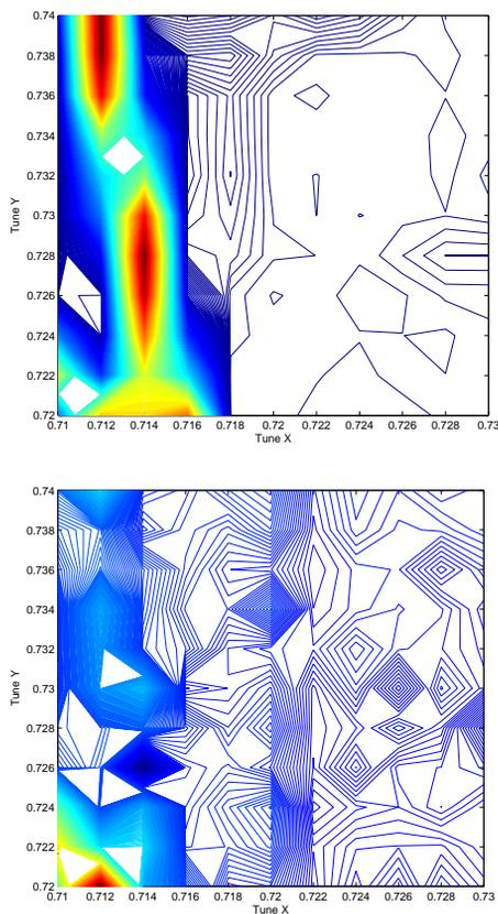
Figure 1: Averaged emittance growth as a function of betatron tunes for 4 sigma and 6 sigma separation including tune modulation.
