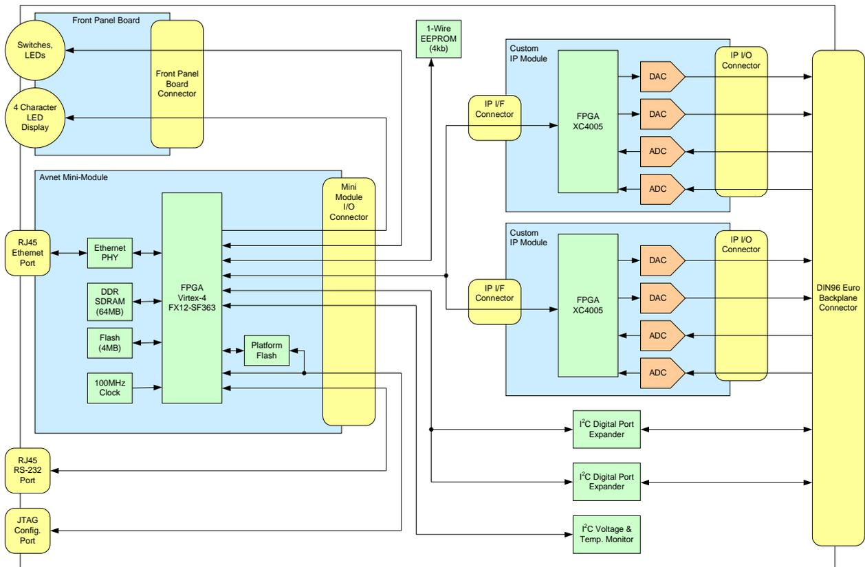
Figure 1: ALS Mini IOC Hardware Block Diagram. The Mini IOC Base Board (outer rectangle) contains connectors for the Avnet Mini-Module, two IndustryPack (IP) Modules and a front panel module.
