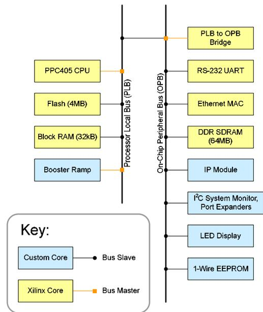
Figure 2: ALS Mini IOC FPGA firmware block diagram.
