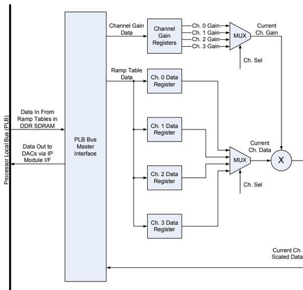
Figure 4: Booster Ramp controller data flow.
