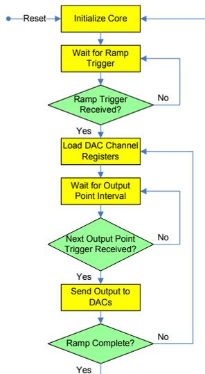
Figure 3: Booster Ramp Controller simplified state machine.
