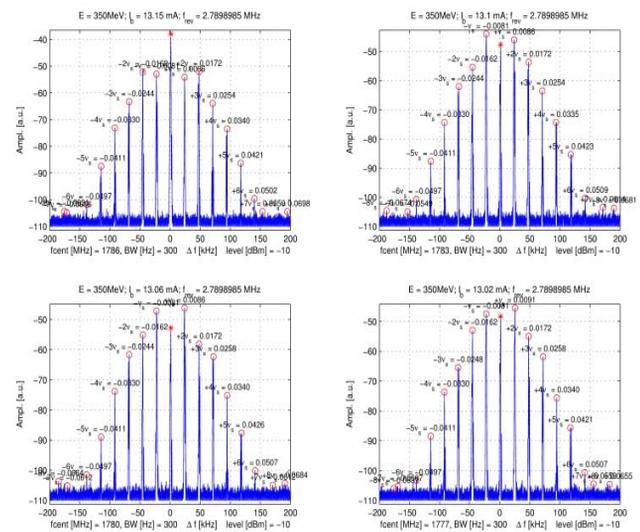
Figure 1: Undamped strong sidebands around a revolution harmonic when beam current was around 13.2 mA at 350 MeV. Here beam is always unstable due to the strong longitudinal CBMIs.
