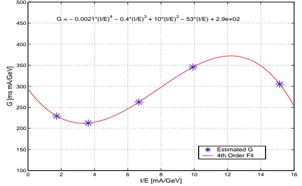
Figure 3: Plot of estimated  $G$  and its 4th order fitting result with respect to  $(I/E)$ .
