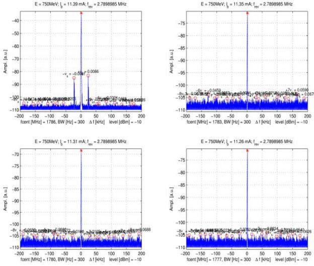
Figure 2: Damped sidebands around a revolution harmonic when beam current was around 11.4 mA at 750 MeV. Here beam is stable if beam current is lower than 11.35 mA at 750 MeV.
