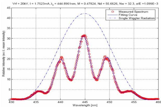
Figure 1: OK-4 spectrum with RF voltage of 20 kV, electron beam current of 1.75 mA, and the fitted energy spread is  $1.1 \times 10^{-3}$ .
