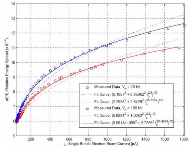
Figure 5: Energy spread vs. single bunch electron beam current for  $V_{rf} = 20$  kV (red) and  $V_{rf} = 100$  kV (blue). Solid curves are fitted with  $\sqrt{\sigma^2 + A^2 I_b^{2/3}}$ , while dash curves are fitted with  $\sqrt{\sigma^2 + A^2 I_b^{2/\alpha}}$ .
