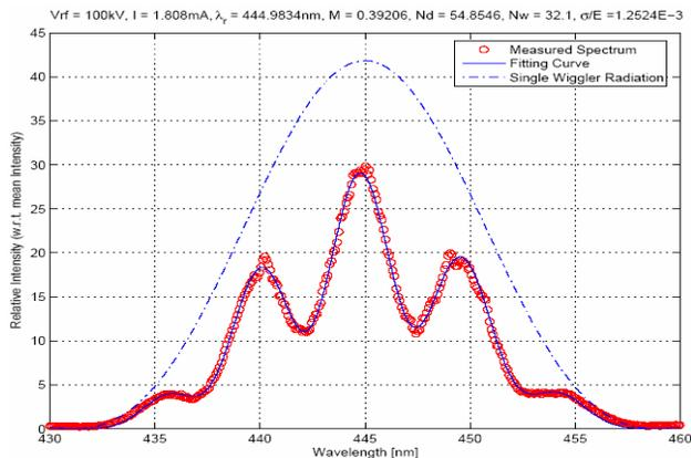
Figure 3: OK-4 spectrum with RF voltage of 100 kV, electron beam current of 1.81 mA, and the fitted energy spread is  $1.3 \times 10^{-3}$ .
