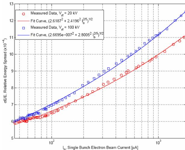
Figure 6: Energy spread vs. single bunch electron beam current for  $V_{rf} = 20$  kV (red) and  $V_{rf} = 100$  kV (blue). Dash curves are fitted with  $\sqrt{\sigma^2 + A^2 I_b^{2/5}}$ .
