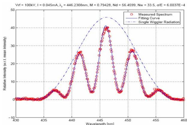
Figure 4: OK-4 spectrum with RF voltage of 100 kV, electron beam current of 0.045 mA, and the fitted energy spread is  $6.0 \times 10^{-4}$ .
