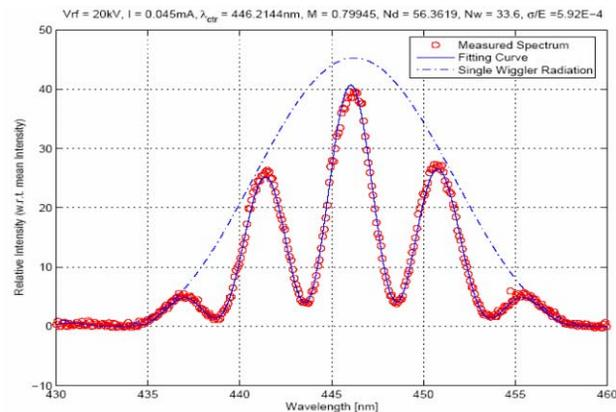
Figure 2: OK-4 spectrum with RF voltage of 20 kV, electron beam current of 0.045 mA, and the fitted energy spread is  $5.9 \times 10^{-4}$ .
