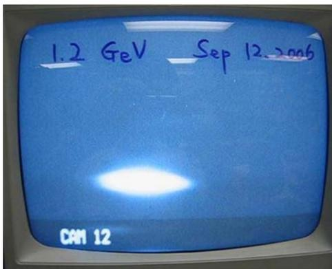
Figure 7. Beam image from SR view port.
