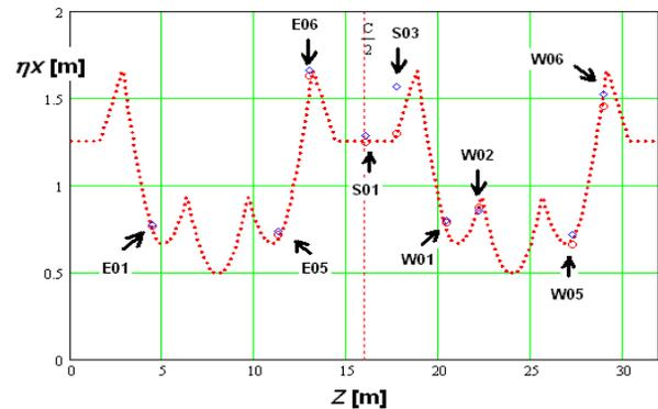
Figure 4. X-dispersion function and BPM measurements.
