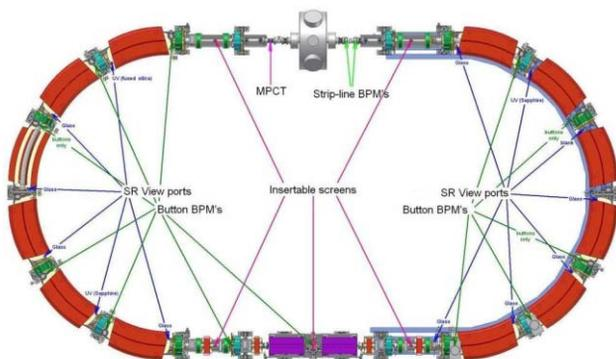
Figure 1. Layout of the main booster diagnostic components.
