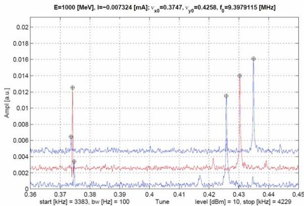
Figure 6. Example of the betatron tune measurements.
