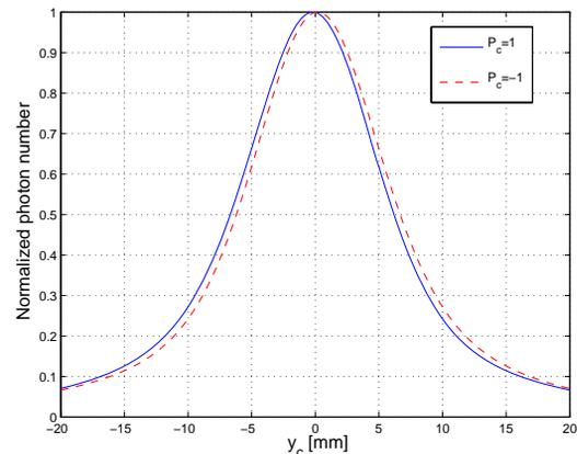
Figure 3: Vertical profiles of scattered gamma-ray photons for 190 nm circularly polarized FEL photons scattering with 1.1 GeV vertically polarized electrons. The solid curve corresponds to the  $P_c = 1$  polarized laser, and the dash curve corresponds to the  $P_c = -1$  polarized laser.
