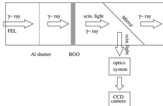
Figure 5: Conceptual design of the gamma-ray imaging system.
