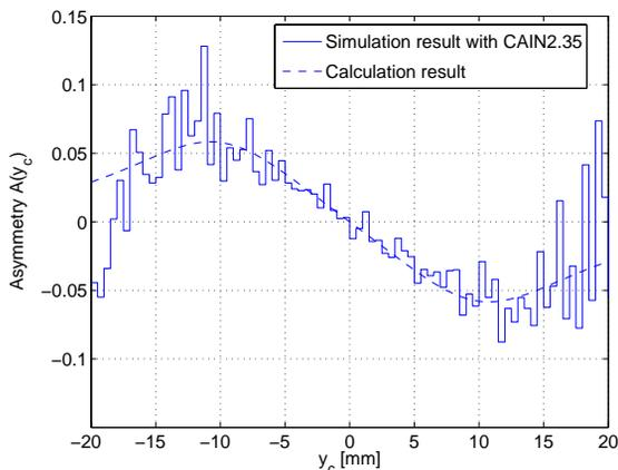
Figure 2: Vertical asymmetry at 30 m from the collision point for 190 nm laser photons scattering with 1.1 GeV electrons. The stairs plot corresponds to the simulation result with CAIN2.35, and the dash curve corresponds to the theoretical calculation.
