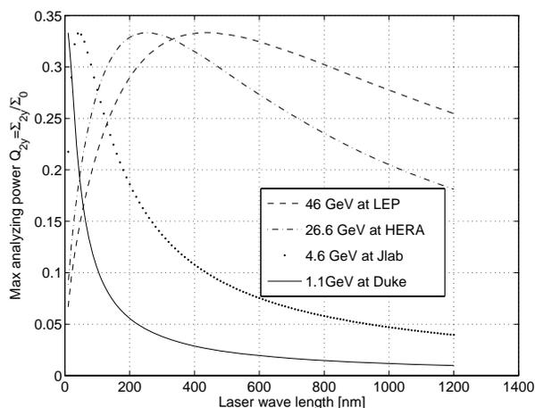
Figure 4: The maximum analyzing power for different electron beam energy and laser wavelength. At the Large Electron-Positron storage ring (LEP) of CERN [5], HERA [4], the Hall A Compton Polarimeter of JLAB [6], and the Duke storage ring, the electron beam energy is 46, 26.6, 4.6 and 1.1 GeV respectively.
