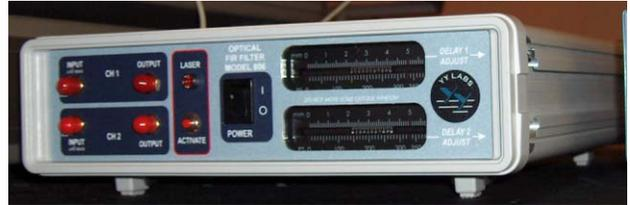
Figure 7: YY-806 optical Notch Filter
