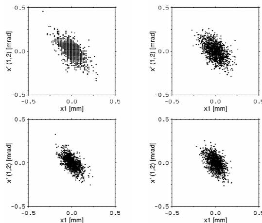
Figure 3: Horizontal beam-centroid coordinates computed from data (left) and from simulation (right), for individual samples (top) and averaged data (bottom) from first and second BPM.
