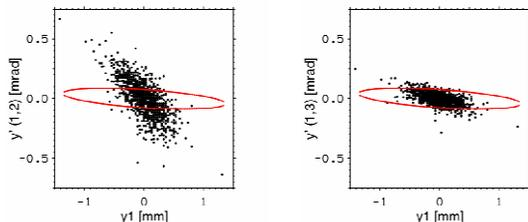
Figure 2: Vertical beam-centroid coordinates at first BPM of 800-MeV H<sup>-</sup> line, computed from data of first two BPMs (left) and from data of first and last BPM (right). The 0.5-rms beam ellipse is shown in red.
