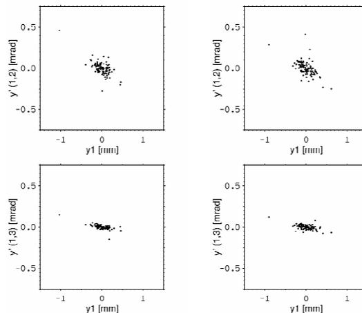
Figure 5: Vertical beam-centroid coordinates computed from data (left) and from simulation (right), for individual samples from first two BPMs (top) and from first and last BPM (bottom).
