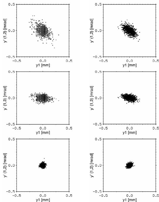
Figure 4: Vertical beam-centroid coordinates computed from data (left) and from simulation (right), for individual samples from first two BPMs (top), individual samples from first and last BPM (middle), and averaged data from first two BPMs (bottom).
