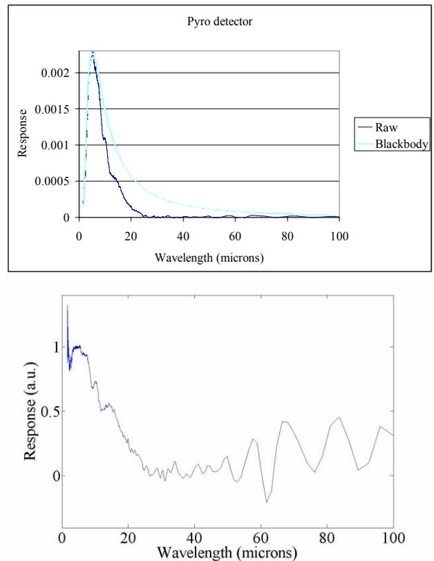
Fig. 2 P1-45 pyrodetector response. (Top) Raw, uncalibrated data with a blackbody radiation spectrum at 993K. (Bottom) Detector response vs. wavelength assuming a source blackbody emission spectra at 993K.
