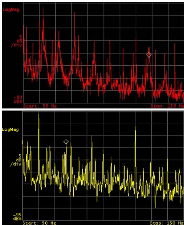
Figure 2. Spectrum of luminosity from 50 to 150 Hz with fast dither on: (a) with support-tube vibration, showing prominent sidebands at  $\pm 9.7$  Hz around dither frequencies (94, 72, and 128) and 60 Hz, and (b) after installing support-tube brace, eliminating sidebands around dither frequencies (93, 77, and 127) and 60 Hz.
