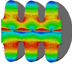
Figure 2: Electric field at a frequency of 3.9 GHz for a 3-cell cavity operating in a  $\pi$  mode in which a wire is displaced 2mm from the electrical centre
