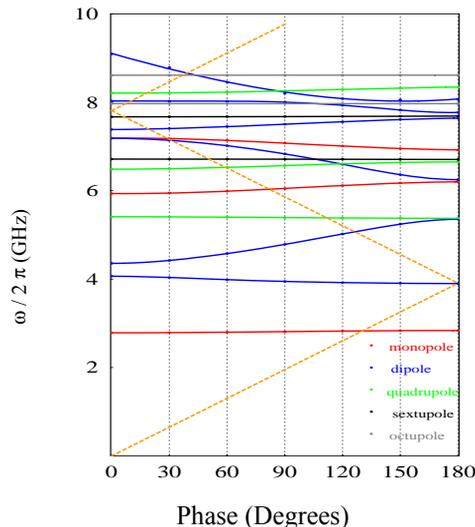
Figure 5: Brillouin diagram for unperturbed cavity
