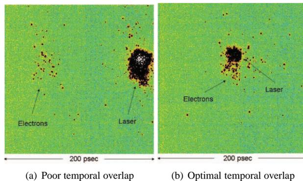
Figure 3: The path length in the laser transport line was adjusted until the faint image from the cherenkov radiation in 3(a) overlapped the clear image from the laser. The result is shown in 3(b). This allows for coarse timing overlap better 50 psec.
