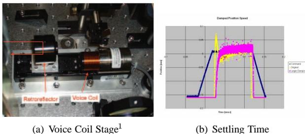
Figure 4: The voice coil controlled translation stage is used to adjust the laser transport path length at a 10 Hz rep rate, with an accuracy of 25 μm (.083 psec), and a range of 30 mm (100 psec).
