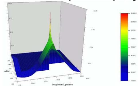
Figure 5: Electric field distribution near a metal corner of a bellows shield finger.
