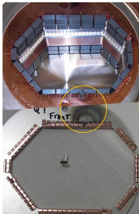
Figure 9: Q2-bellows and Ω-seal with traces of sparking.
