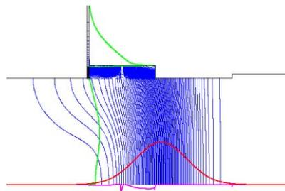
Figure 2: Simulation model. Electric displacement force lines.
