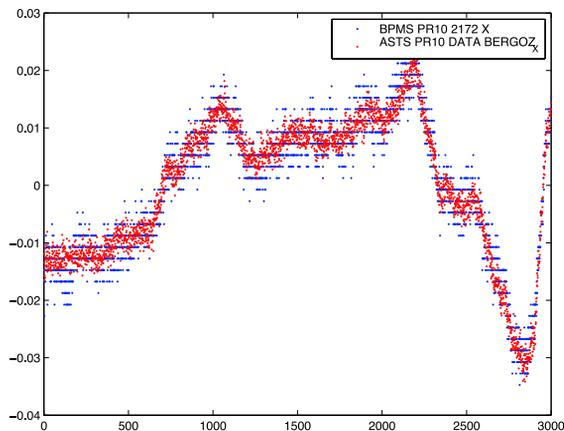
Figure 2: Correlation plot data comparing the position horizontal position reading from the BERGOZ module to the PEP II unit. The BERGOZ unit is scaled and offset corrected, since it was set for SPEAR. The blue trace shows the PEP and the red the BERGOZ unit.
