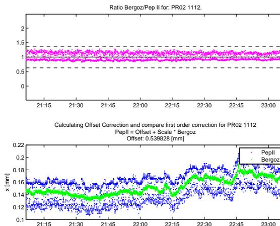
Figure 4: Correlation plot results for the units installed in location PR02 1112 in the LER for the horizontal plane. The upper plot shows the ratio of the BERGOZ position measurement to the PEP. The lower shows the actual position readings with the BERGOZ units (green trace) with offset corrected. The PEP unit's (blue trace) position readings depicts a two state behavior which is unphysical.
