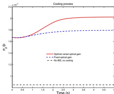
Figure 3. Energy spread variations during cooling.
