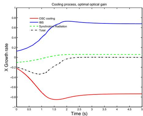
Figure 2. The  $\frac{1}{2}$  transverse growth rates during cooling.
