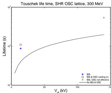
Figure 5. Touschek lifetime vs.  $V_{rf}$ .
