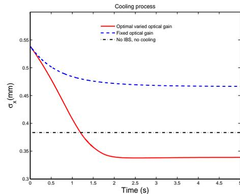
Figure 1. Transverse beam size reduction due to OSC.
