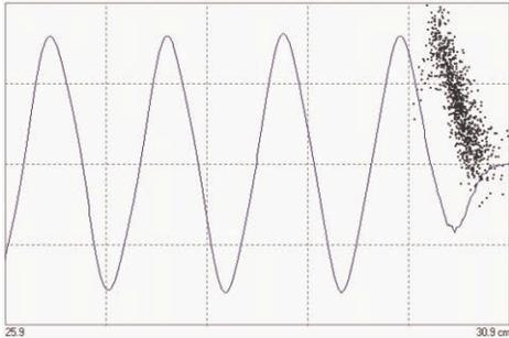
Figure 1: Beam breakup simulation for the 26 GHz power extractor using DWA-BD-02. (15 MeV, 20 nC beam, 1.5 mm rms length, 0.1 mm initial offset,  $E_z \sim 18$  MV/m).
