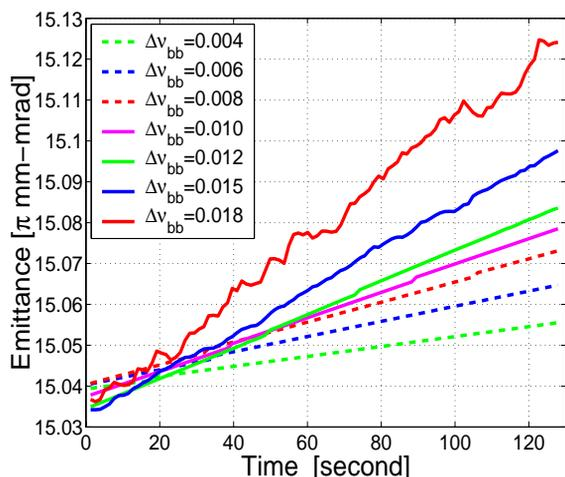
Figure 1. Emittance evolution of beams with different beam-beam parameters as function of time.
