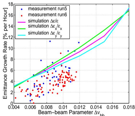
Figure 2. The emittance growth rate from the simulation compared to the measured beam emittance growth of early 4 hours in RHIC stores during Run 2005 and Run 2006 as function of beam-beam parameter.
