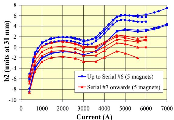
Figure 1: Normal sextupole (integral value) as a function of magnet current in the D0 dipoles.
