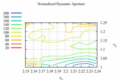
Figure 5: Tune Scan of Optimized DA (normalized with  $\sqrt{\beta_x \beta_y}$ , using pseudo-invariant).
