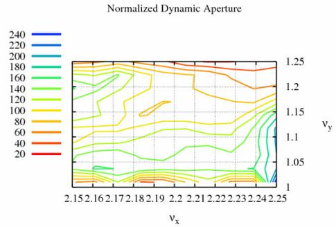
Figure 4: Tune Scan of Optimized DA (normalized with  $\sqrt{\beta_x \beta_y}$ , using Lie Generator).
