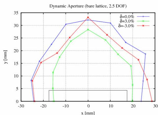
Figure 7: Dynamic Aperture for  $\delta=0$  and  $\pm 3\%$ .
