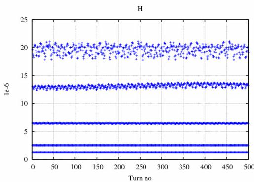
Figure 3: Variation of the 5<sup>th</sup> Order Pseudo-Invariant on a Turn-by-Turn Basis.
