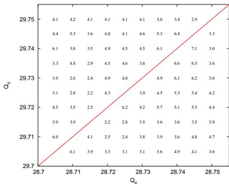
Figure 5: DAs in the tune scan above 0.7 under condition of (IRerrcorr + BB + b2 + 2fam ).
