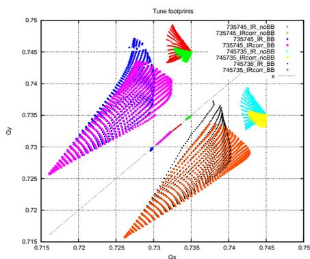
Figure 2: Above 0.7: The tune footprints with and without IR multipoles corrections for on-momentum particles up to  $6\sigma_0$ . The tune spots on the diagonal are due to the failure in tune searching.
