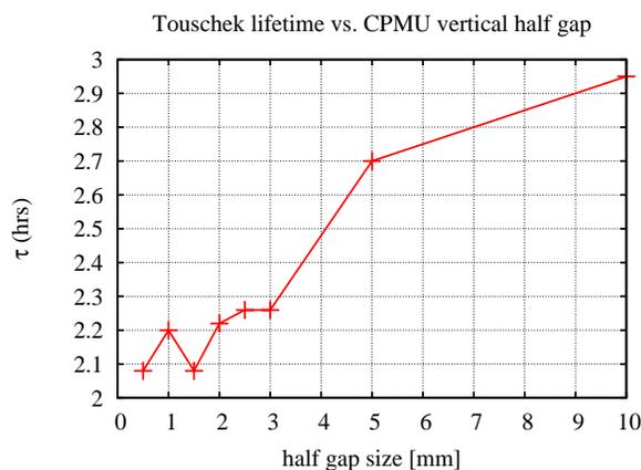
Figure 6: Touschek lifetime in NSLS-II for varying vertical gap size in CPMUs.
