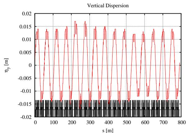
Figure 2: Vertical dispersion wave around the ring.
