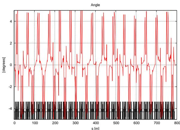
Figure 4: Transverse coupling angle around the ring.
