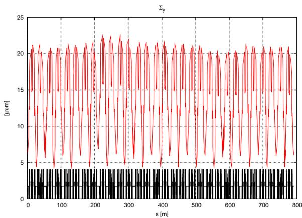
Figure 3: Vertical beam size around the ring.
