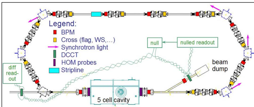
Figure 2: L layout of ERL Recirculation Loop Diagnostics.
