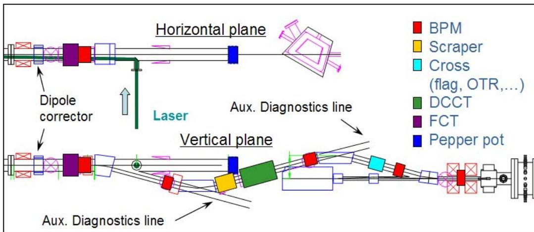
Figure 1: L layout of ERL Injector Diagnostics.
