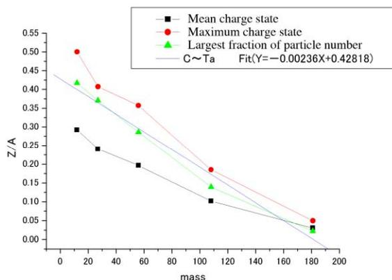
Figure 5: Charge states using the Nd-YAG laser.
