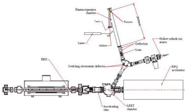
Figure 12: Floor layout plan for the LIS + EBIS.
