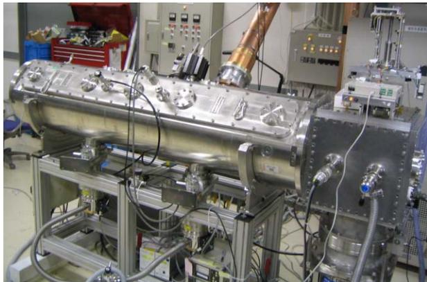
Figure 7: 100MHz 4-rod RFQ with DPIS-LIS.
