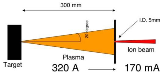
Figure 1: Ion beam current extracted from laser plasma.
