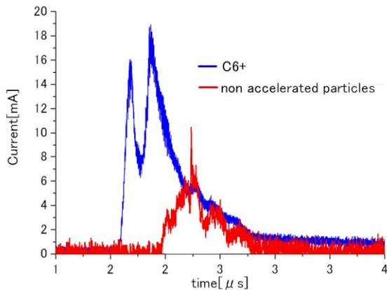
Figure 9: Fully stripped carbon beam acceleration.
