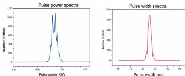
Figure 3: Stability of the 100 J CO<sub>2</sub> laser in generator mode.
