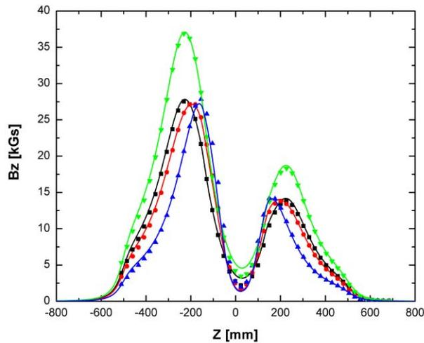
Figure 5. Axial magnetic field profiles at  $r=55.9$  mm radius. Solid lines – calculated, dots – measured. Green – 24 GHz (390, 0, -66, -66, 0, 280 A); black – 18 GHz (290, 0, -50, -50, 0, 210 A); red – 18 GHz (175, 175, -130, -130, 135, 135 A); blue – 18 GHz (0, 390, -220, -220, 320, 0 A)
