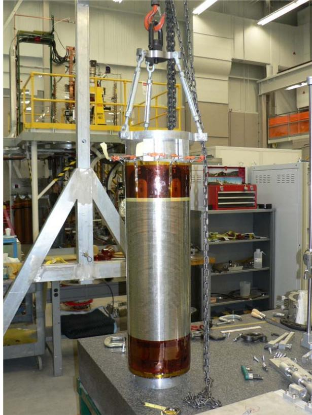
Figure 1. The banded hexapole coil assembly ready for insertion in the solenoid bobbin bore.
