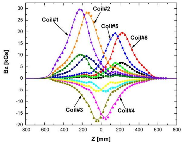
Figure 4. Axial magnetic field profiles of the individual coils excited with 100 and 300 A currents. The field values were measured at r=55.9 mm radius and 0 degrees. Solid lines – calculated, dots – measured.
