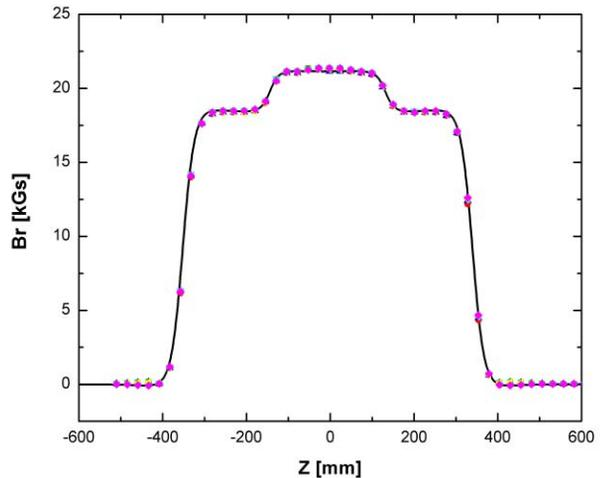
Figure 3. Radial magnetic field measured parallel with the plasma chamber axis at r=56.2 mm radius. Solid line – calculated; colored dots – measured values at 0, 60, 120, 180, 240 and 300 degrees.
