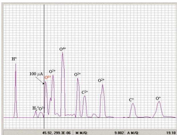
Figure 6. Oxygen charge state distribution. The 18 GHz microwave power was 150 W, 15 kV extraction voltage.
