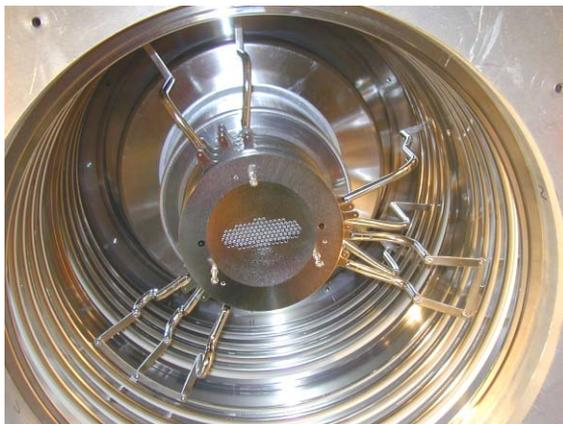
Figure 5: Einzel Lens Assembly for the Merging Experiment installed in the top of the column (without the field shield installed).
