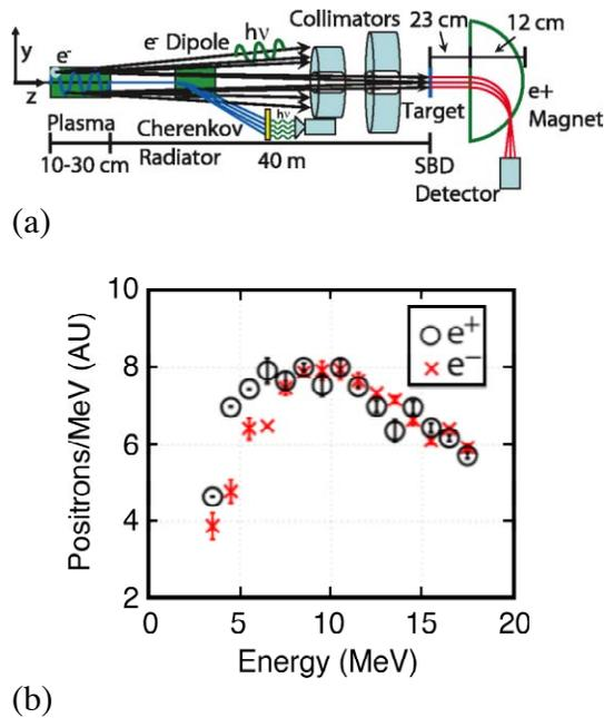
Figure 4. (a) Schematic set-up for the utilization of betatron x-rays for pair-production and (b) both  $e^+$  and  $e^-$  spectra measured for the same plasma and beam conditions.
