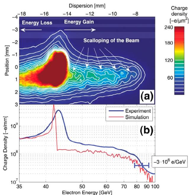
Figure 1. (a) The energy spectrum of the (initially nominally 42 GeV) electron beam after passage through an 85 cm long,  $2.7 \times 10^{17} \text{ cm}^{-3}$  Lithium plasma and (b) a comparison between the measured spectrum and the simulated spectrum. Reprinted by permission from Macmillan Publishers Ltd: *Nature* 445, 741-744, © 2007.
