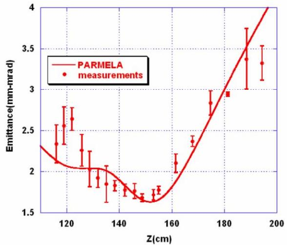
Figure 3: Emittance evolution, “flat top” case, measurements and PARMELA simulations
