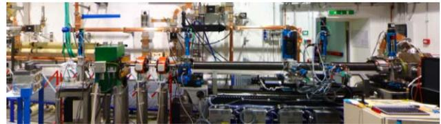
Figure 1: Picture of the SPARC photoinjector showing the RF gun with its solenoid (right end) the emittance meter (centre), the energy spectrometer and the beam dump (left end).
