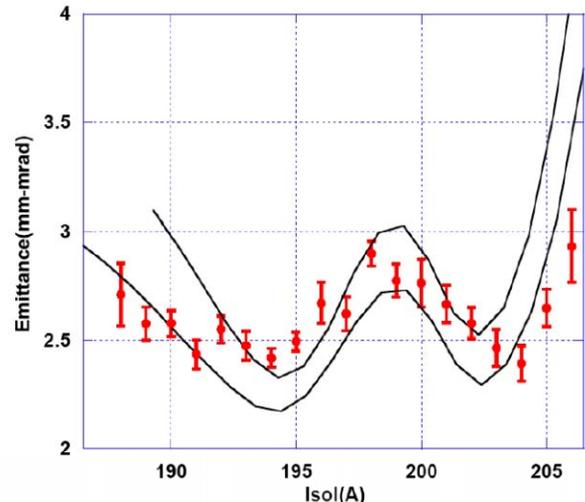
Figure 7: Emittance versus solenoid magnetic field at a fixed position ( $z=150$  cm). Same beam of fig. 5. Simulations with charge fluctuations of 6 % are shown.
