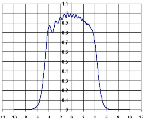
Figure 2: “Flat top” temporal laser pulse shape with 8.9 ps FWHM and 2.6 ps rise time.
