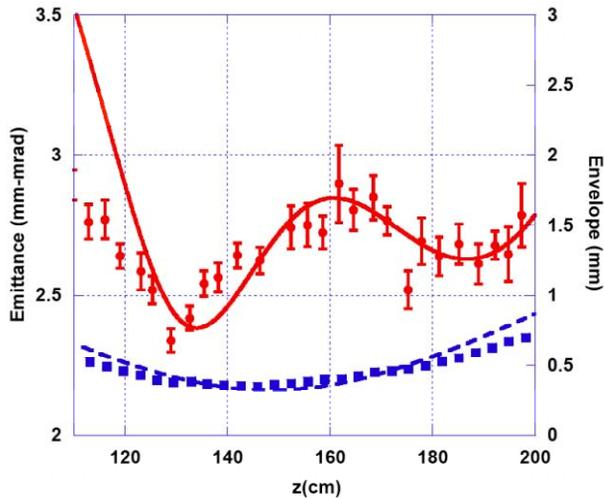
Figure 5: Envelope and Emittance downstream the RF gun of a “flat top” bunch.
