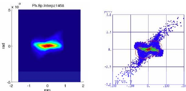
Figure 6: Transverse phase space at  $z=150$  cm. Same beam of fig. 5
