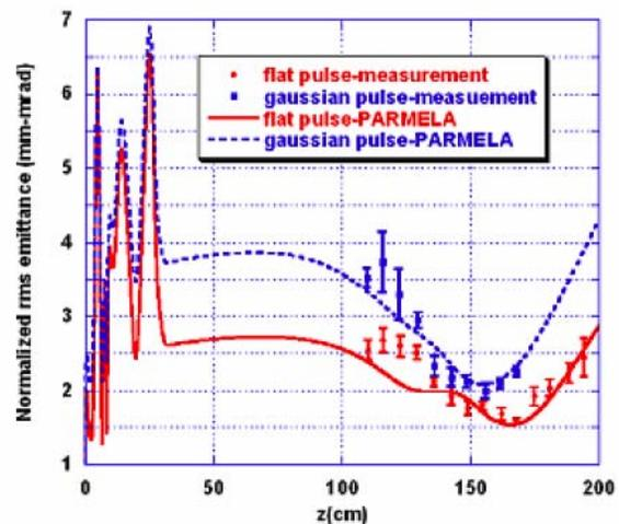
Figure 4 : Emittance evolution of Gaussian and “flat top” beams. Measurements and PARMELA simulations.
