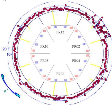
Figure 1: Temperature rise in the LER quad chambers due to rf voltage change from 4.05 MV to 5.6 MV.
