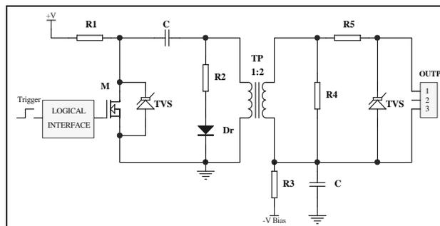
Figure 3: Block diagram of the thyatron driver
