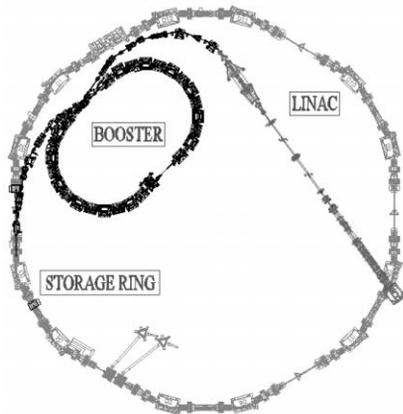
Figure 1: Layout of the LNLS light source, showing the 120 MeV injector LINAC, the 500 MeV booster synchrotron and the 1.37 GeV storage ring.
