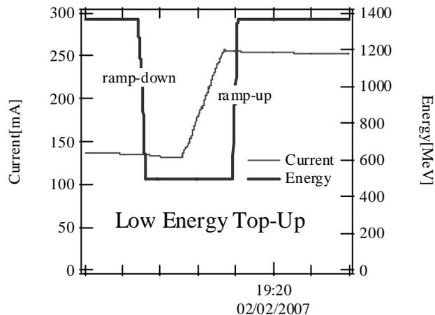
Figure 5: Low energy topping-up of the current at the LNLS storage ring.
