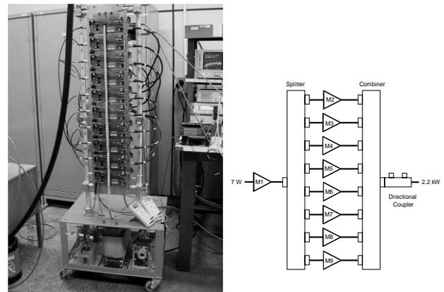
Figure 7: Amplifier assembly and block diagram.
