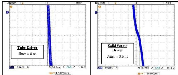
Figure 4: Modulator jitter measurement before (left) and after (right) the replacement of low power thyratron tubes with a solid-state driver.
