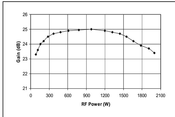
Figure 6: Gain response of the 476 MHz, 2.2 kW CW amplifier.
