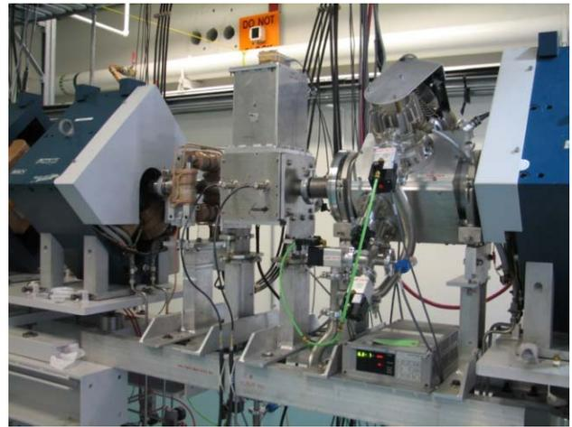
Figure 4: The monitor installed in the beamline downstream of the SC-linac at SEBT:DB18B.
