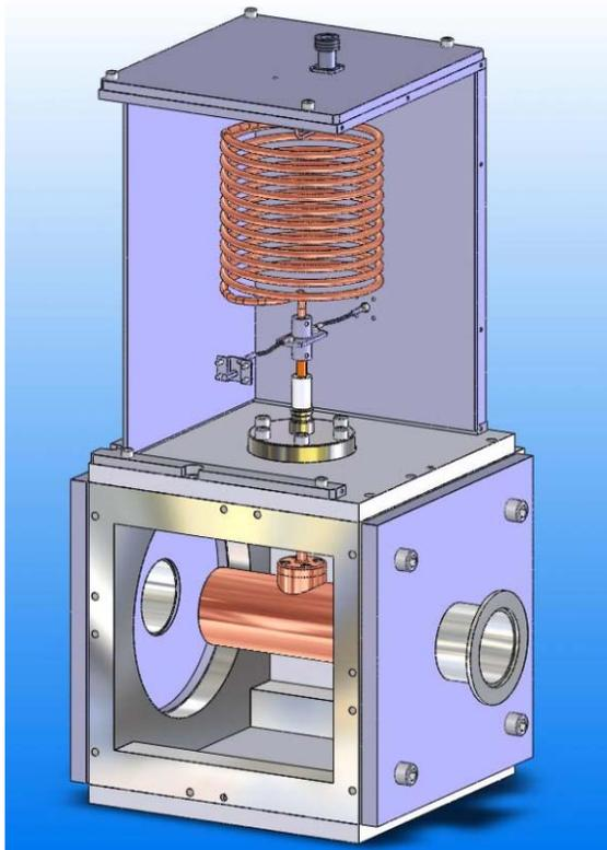
Figure 1: A SolidWorks drawing of the monitor showing the pickup tube and helical resonator.
