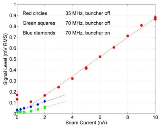
Figure 3: The sensitivity tested in the double s-bend transfer line, with straight line fits.
