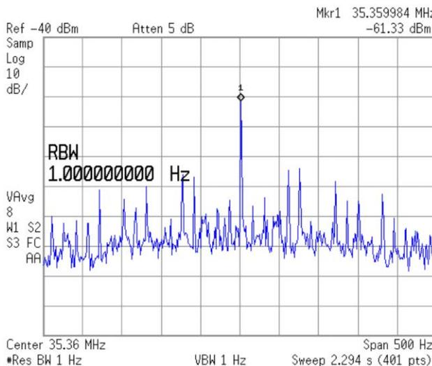
Figure 6: The spectrum of a 3.5 nA  $^{22}\text{Ne}^{+4}$  beam at 3.6 MeV/u.
