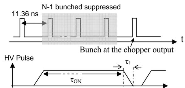
Figure 1: Beam structure and Chopping time structure.
