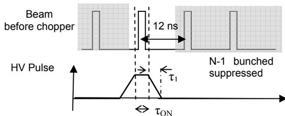
Figure 4: high voltage pulse with inverted duty cycle.
