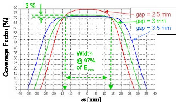
Figure 6: Transverse coverage factor on the beam path.
