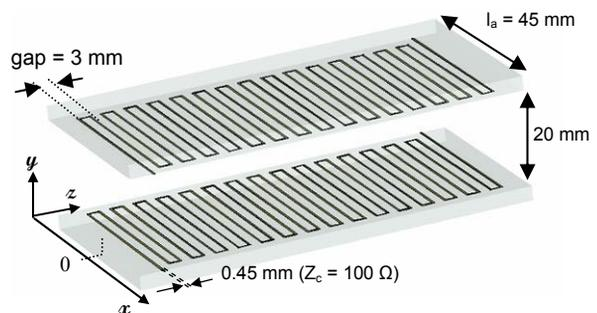
Figure 5: Design of the 100-Ω meander line.
