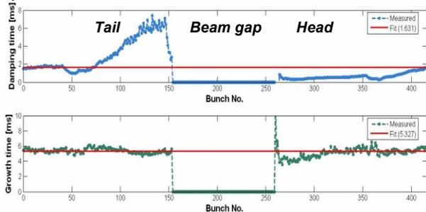
Figures 6: Observed bunch by bunch feedback damping and instability growth times at 50 mA in 3/4<sup>th</sup> filling.
