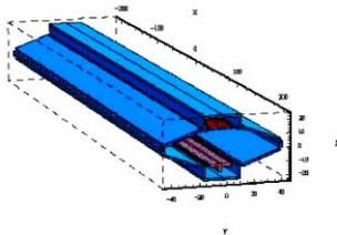
Figure 3: Vertical stripline with 2 electrodes.
