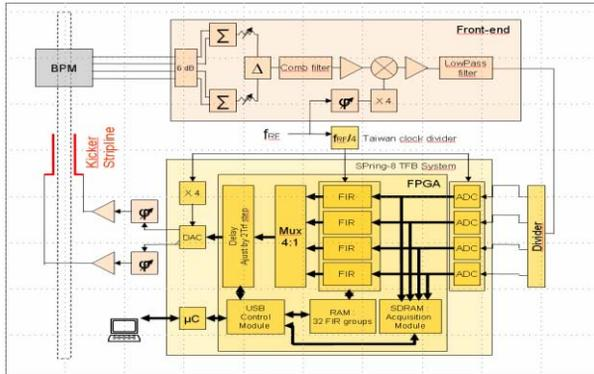
Figure 2: Layout of the SOLEIL feedback chain.
