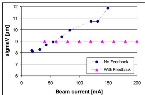
Figure 7: Vertical beam size versus current measured with a pinhole camera [5] at a non-zero chromaticity.
