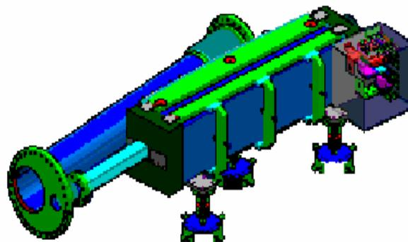
Figure 1: Sketch of the new inflector magnet (right) next to the SIS18 beam pipe (left).
