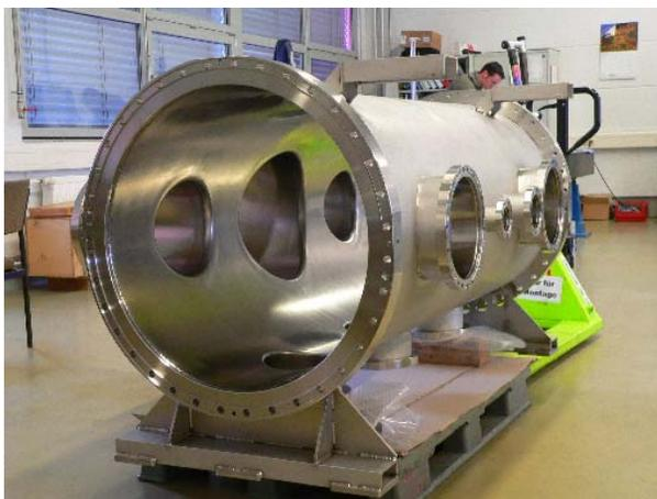
Figure 2: Electrostatic septum tank after manufacturing.
