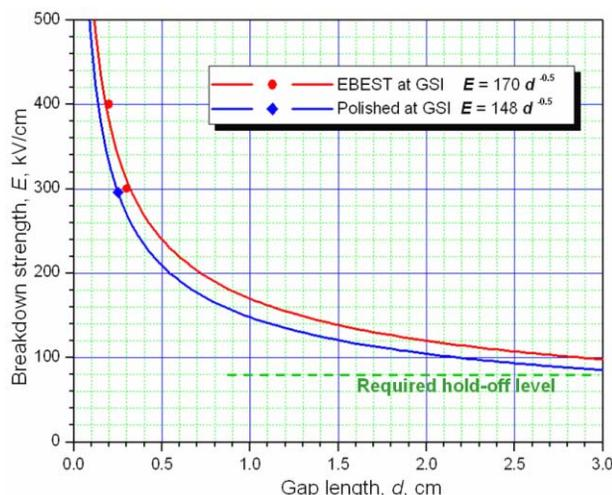
Figure 4: Results of DC breakdown tests for small-sized HV-gaps treated with different polishing techniques.
