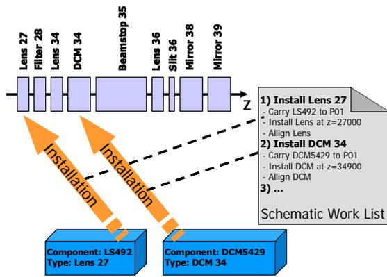
Figure 6 Installation of components in reserved slots.
