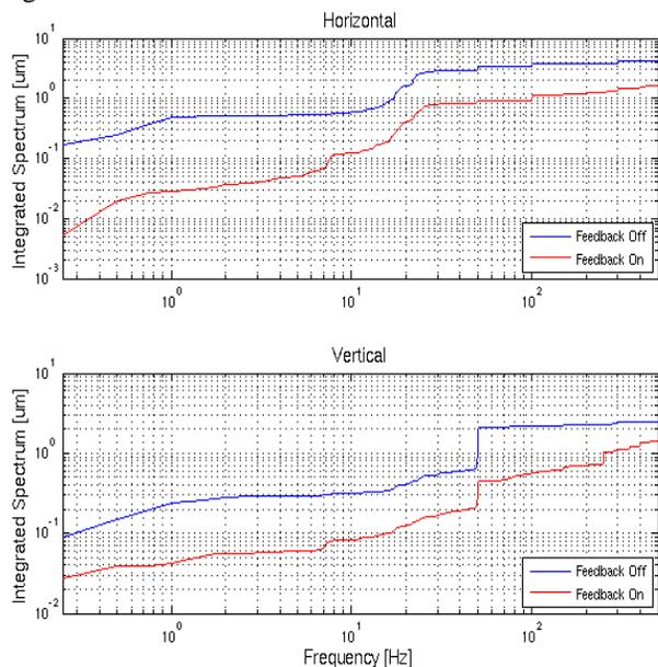
Figure 4: Integrated amplitude spectrum of the beam position noise measured by a BPM with feedback off (blue line) and on (red line).
