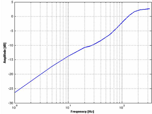
Figure 2: Measured closed loop transfer function (sensitivity function) showing the attenuation of noise components as a function of frequency.
