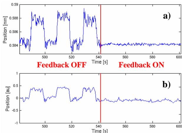
Figure 5: Effect of the feedback in the vertical plane measured by an electron (a) and a photon (b) BPM. The beam orbit is perturbed by the operation of the electromagnetic elliptical wiggler.
