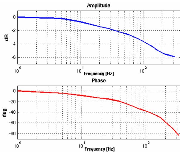
Figure 1: Amplitude and phase response of a corrector magnet measured by exciting it with sinus waves at different frequencies.
