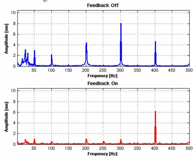
Figure 3: Amplitude spectrum of the horizontal beam position with feedback off and on. The loop is closed with a PID regulator and four harmonic suppressors at 50, 100, 200 and 300 Hz.
