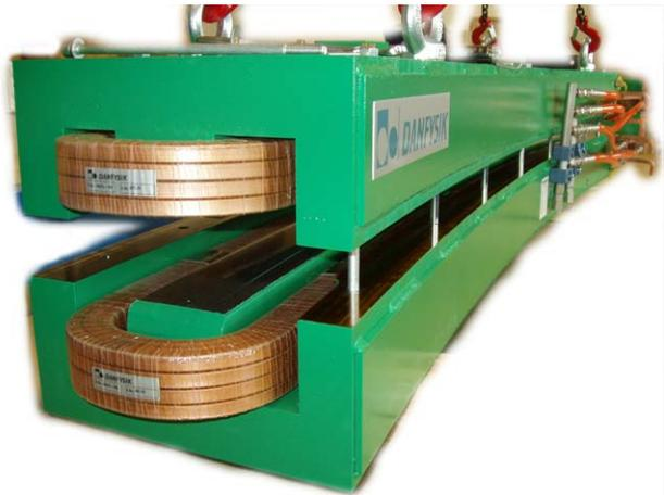
Figure 1: Dipole during vacuum chamber installation
