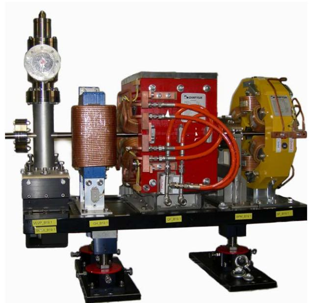
Figure 2: Horizontal steerer, focussing quadrupole and sextupole magnets assembled on the girder
